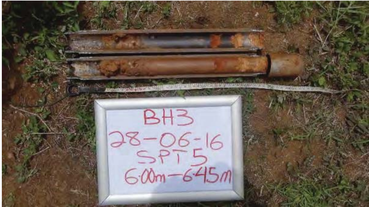
Plate 6 : SPT showing reddish brown light yellowish silty clayey sand with lateralized gravel.
