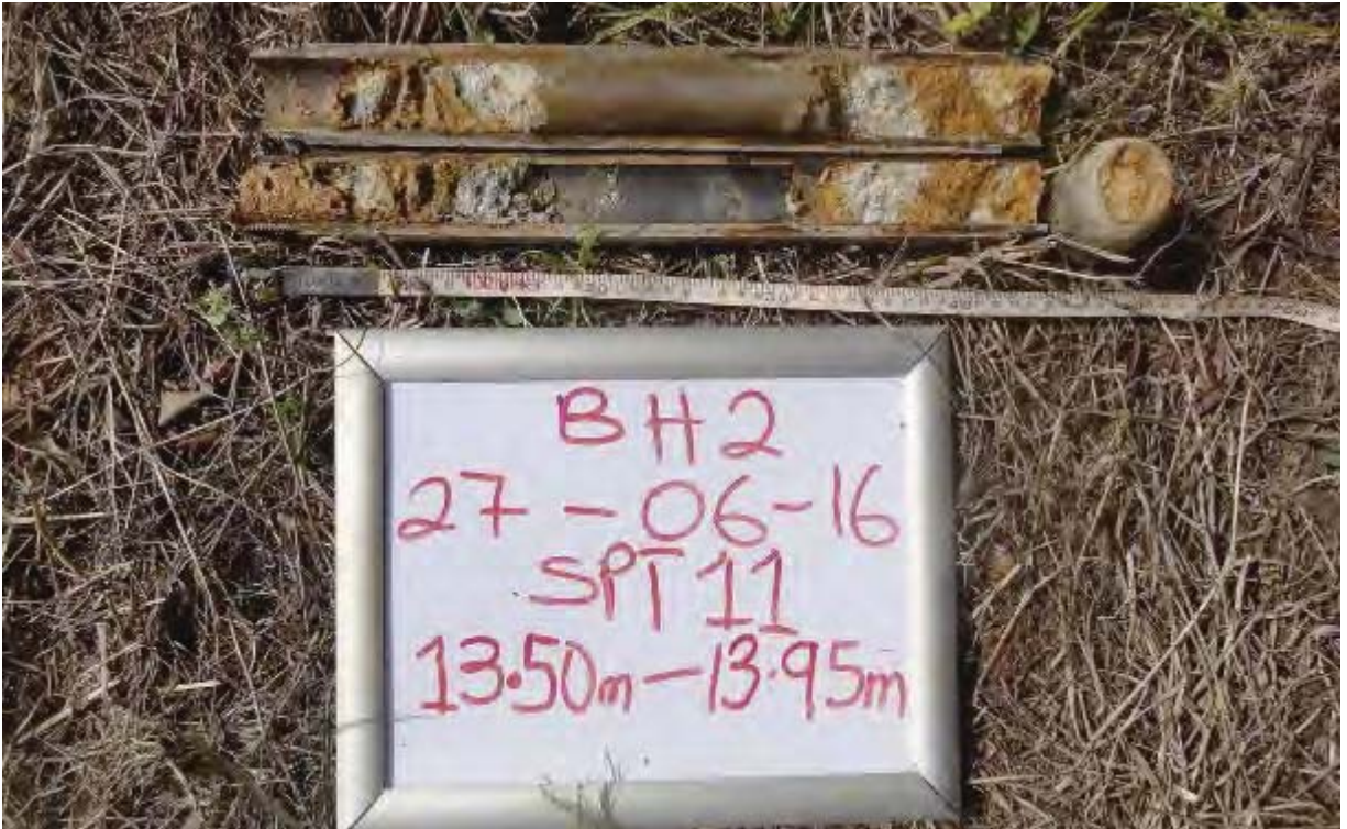
Plate 7: SPT showing Light yellow grey-greenish silty sandy clay with decomposed rock fragments
